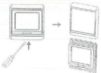
Take the backing plate apart according to the following diagram.
