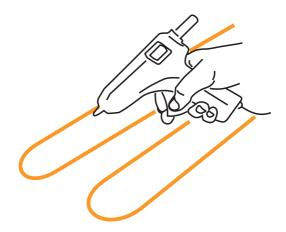
Note: The temperature sensor has to be placed at an equal distance between heating cables.
