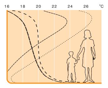
Vertical temperature distribution within the room for various types of heating.
